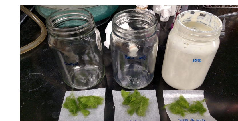
Algae sample preparation using titanium dioxide-painted glassware.
